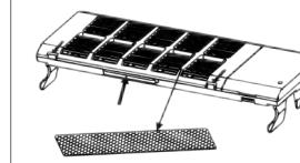
Releasing the buckles as indicated with arrows and open the cover of the Plasma, clean or replace the filter with vacuum.
